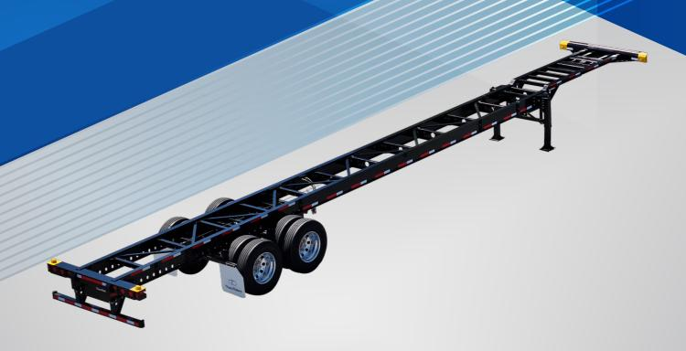
Retracted Length Overall Width Overall Height Payload Tare Weight 53'7" 96" 55" 67,200 lbs 7,450 lbs
