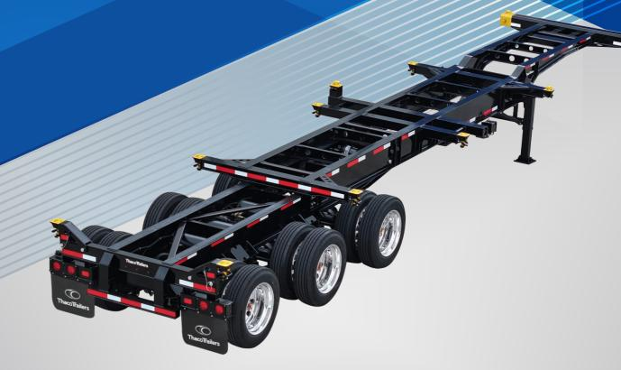
Retracted Length | Extended Length | Overall Width | Payload 20' | Payload 40' | Tare Weight 31'7" | 40'11" | 96" | 66,100 lbs | 74,100 lbs | 10,900 lbs
