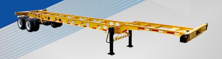
Overall LengthOverall WidthOverall HeightPayloadTare Weight40' 11"96"58"67,200 lbs5,250 lbs
