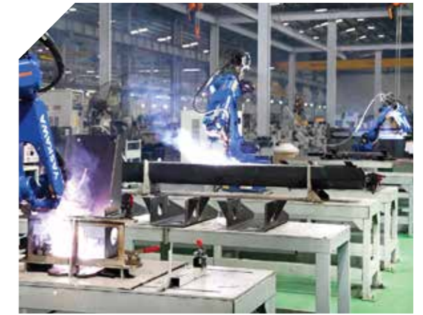
3 Front bolster and rear bolster welding
