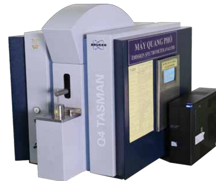
Spectrograph machine (material composition testing)
