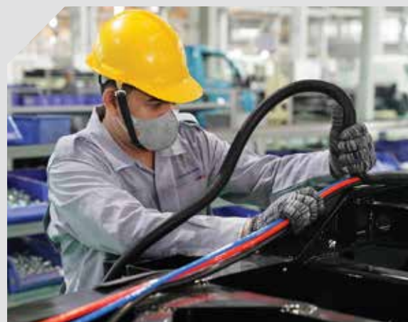
2 Electrical system assembly
