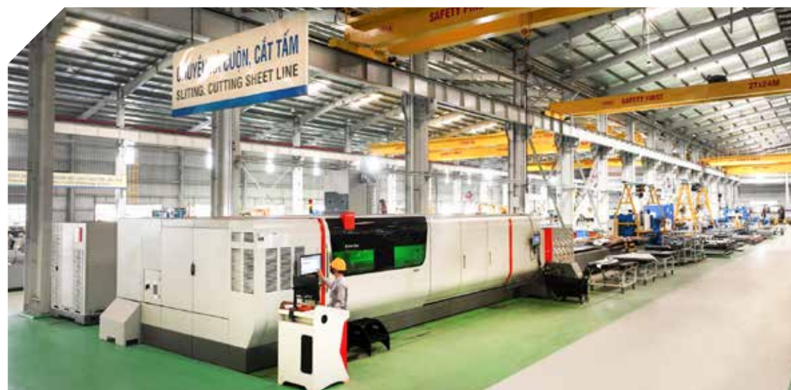
MÁY CẮT FIBER LASER FIBER LASER CUTTING MACHINE
