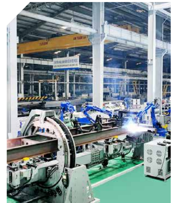
4 HÀN ROBOT CHASSIS WELDING ROBOT
