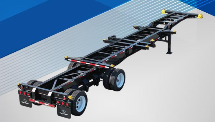
Retracted Length | Extended Length | Overall Width | Payload 20' | Payload 40' | Tare Weight 31'7" | 40'11" | 96" | 54,500 lbs | 57,000 lbs | 9,350 lbs
