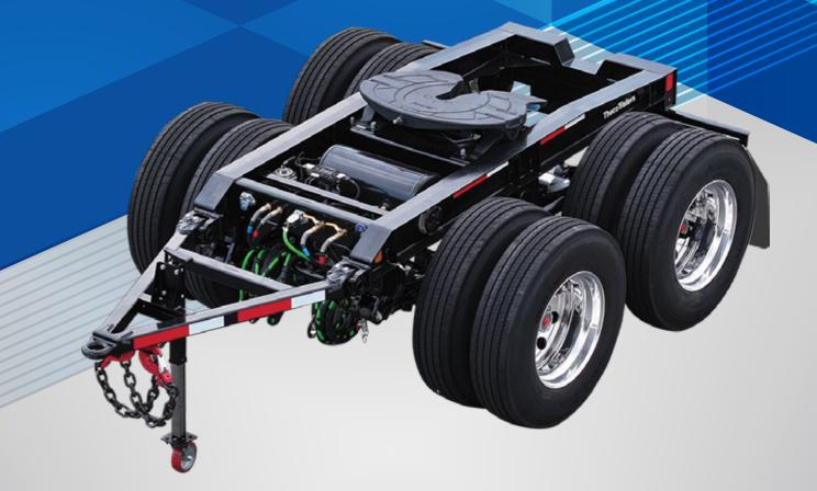
Overall Length Overall Width Axle Spread Tare Weight GVWR 13' 5" 49" 4,800 lbs 44,000 lbs
