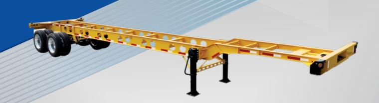
Overall Length Overall Width Overall Height Payload Tare Weight 40' 11" 58" 67,200 lbs 5,250 lbs
